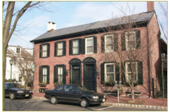
Federal Style, 1800—1840. This early style typically features a low-pitched roof, simple, symmetrical box-like exterior, and sidelights or windows surrounding the front door.
