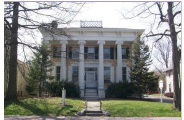
Greek Revival, 1820—1860. The large massive columns and pedimented porches are the signature of this style, reminiscent of ancient Greece's monumental buildings.
